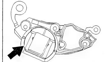
DISMANTLING AND CHECKING ALTERNATOR Checking (installed) rectifier
